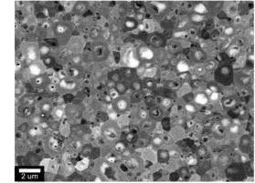
Figure 2 – Highly contrasted backscatter scanning electron microscopy image revealing chemical heterogeneity in 20Bi(Zn<sub>0.5</sub>Ti<sub>0.5</sub>)O<sub>3</sub>-80BaTiO<sub>3</sub> ceramics.
