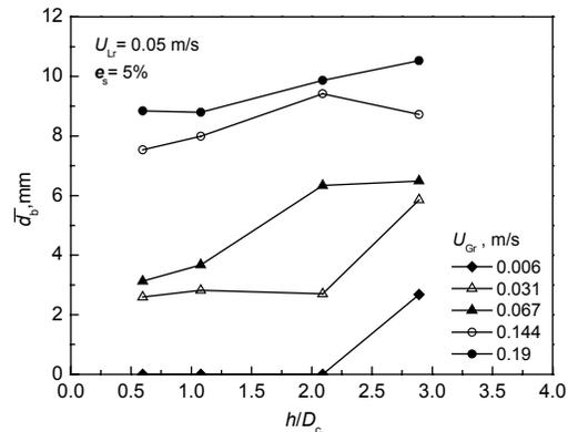
Fig.4 The axial variation of cross-sectional average bubble size in the annulus
