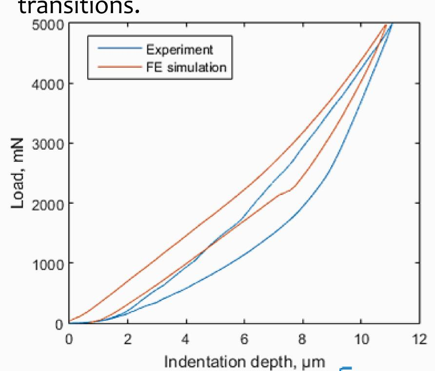
Comparison between FE simulations and indentation experiment for 55.1 Ni 44.9 Ti
