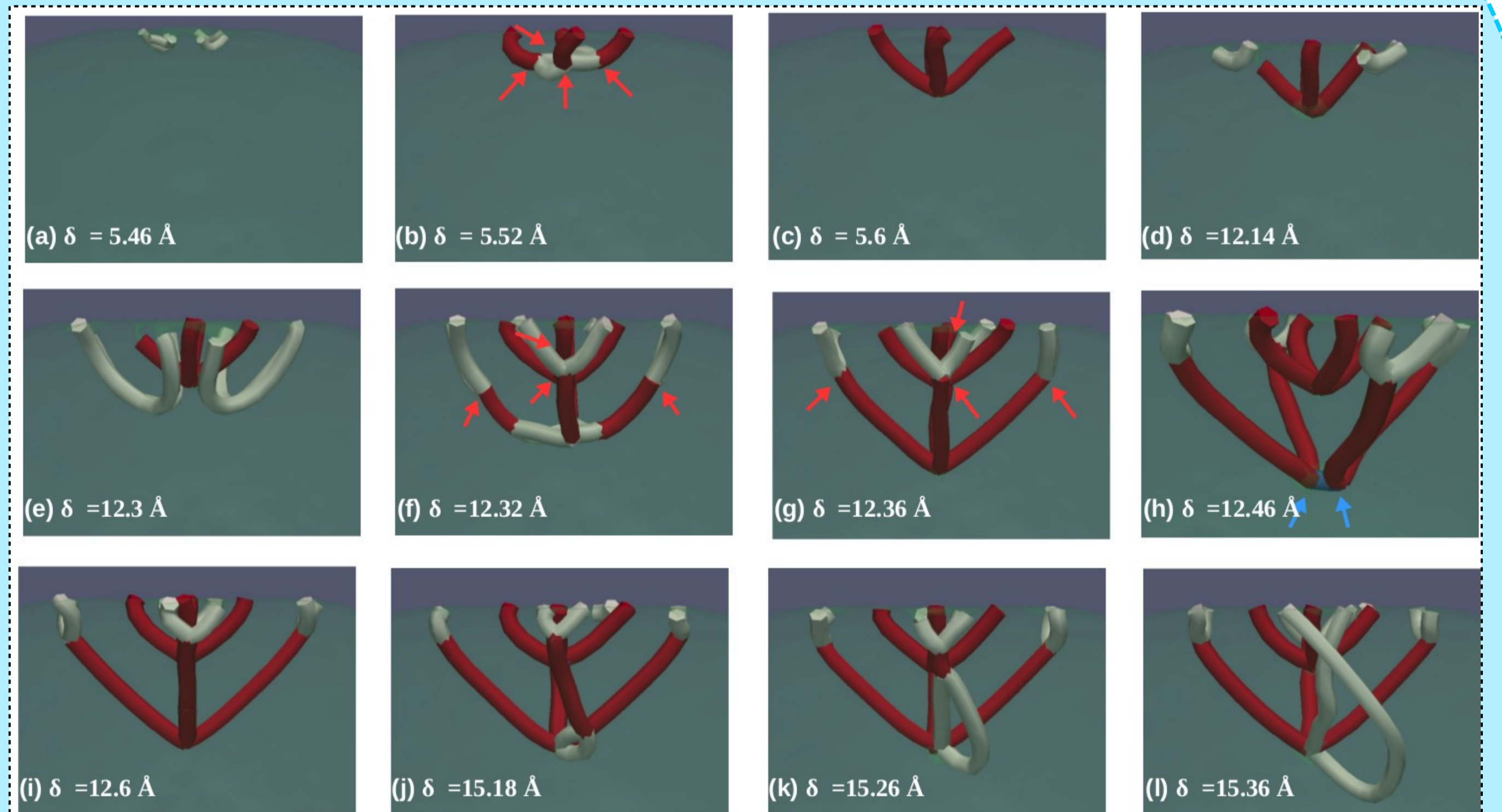
Visualization of the evolution of dislocation structures during plastic deformation (Visualization using ParaView): white line, Shockley partial dislocation with Burgers vectors 1/6 \langle 112 \rangle ; red line, stair-rod dislocation with Burgers vectors 1/3 \langle 100 \rangle and blue line, stair-rod dislocation with Burgers vectors 1/3 \langle 110 \rangle .
