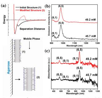
Figure 2 – Selective adsorption to hydrogels. (a) Entropic differences to the surfactant structure effects the potential energy between the SWCNT and substrate. High-fidelity separations of the (6,5) nanotube as characterized by (b) fluorescence and (c) absorbance spectroscopy. Note that the absorbance spectra show the first and second energy transitions.
