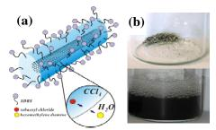
Figure 1 – (a) Coating SWCNTs through interfacial polymerization. (b) Encapsulated SWCNT product freeze-dried and re-dispersed.
