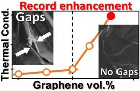
Figure 1 – Thermal conductivity enhancement via gap closure between adjacent fillers
