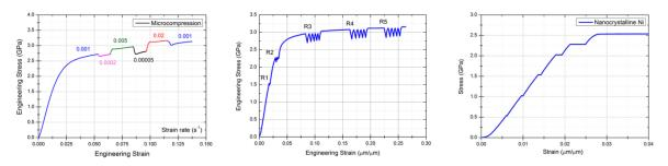
Figure 1. Strain rate jump, stress relaxation and creep tests on nanocrystalline Ni micropillars at room temperature
