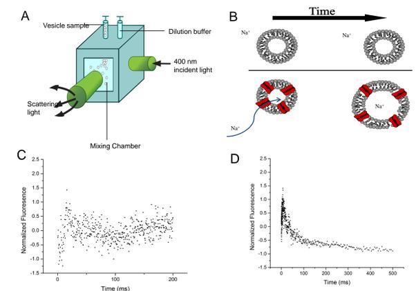
Figure 4. (A) Schematic representation of stopped flow spectrophotometer. (B) Comparing vesicles in the mixing chamber with respect to time. NaChBac vesicles swells once Na<sup>+</sup> enters the vesicles and causing its buffer to become hypotonic. (C) The scattering light detected with respect to time when 100 nm diameter liposomes enter NaCl buffer. (D) The scattering light detected with respect to time when 100 nm diameter NaChBac vesicles mix with the NaCl buffer.
