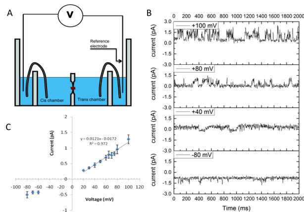
Figure 1. (A) A schematic representation of the planar lipid bilayer device used to study NaChBac. (B) Single channel recordings at different holding potentials. (C) Average peak current (I-V) plots.
