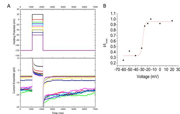
Figure 3. (A) Current ensembles for various voltage-clamp protocols. (B) Normalized activation curve and fitted using the Boltzmann equation which is shown in Equation (3).
