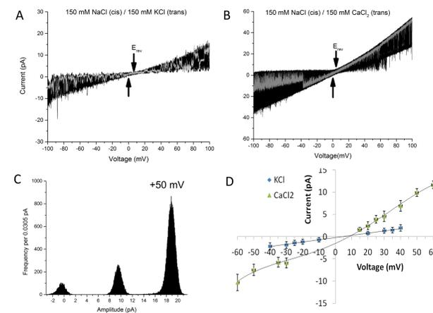
Figure 2. Relative permeability of NaChBac. 100 voltage ramp sweeps at 100mV/s are recorded and for (A) KCl and (B) CaCl<sub>2</sub> biionic conditions. 1 of the 100 sweeps is highlighted in gray for ease of viewing. (C) All point current histogram for CaCl<sub>2</sub> biionic conditions. (D) Conductance curves for KCl and CaCl<sub>2</sub> biionic conditions.
