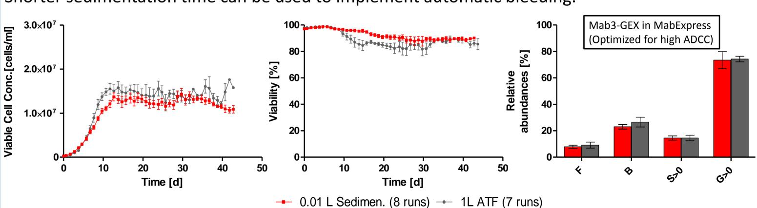
Down scale cultivations are in very good agreement with 1 L ATF cultivations. Viability for sedimentation based perfusion is higher than for ATF cultivations. Up to eight times of stirring and pH-DO control stop for 40 minutes does not negatively impact growth and viability. Glycan structures are highly comparable to larger scale cultivations (see figure on the lower left for more glycosylation data).
