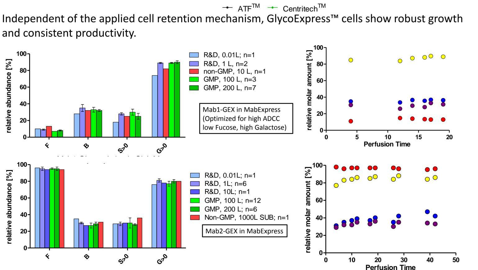
No measurable differences in product quality between batches, batch sizes, reactor sizes, process control strategies, DSP scales and production site. Glycan structure analysis was performed by Instant AB™ labelling and HPLC-MS.
