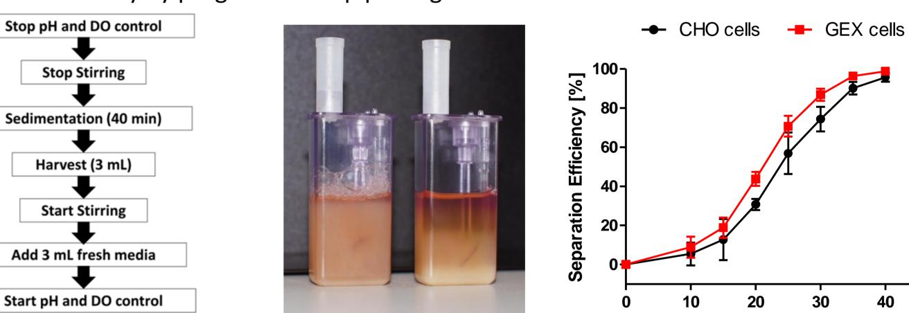
40 minutes are sufficient to achieve a separation efficiency of >99% for GEX and CHO cells. Shorter sedimentation time can be used to implement automatic bleeding.
