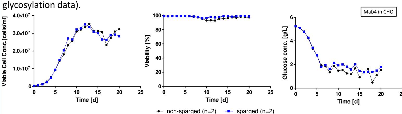
The sedimentation based ambr perfusion is applicable to CHO as well. CHO cells show good growth and high viability independent of the aeration strategy for a non-optimized perfusion process. Data for larger scale CHO perfusion is not available yet.
