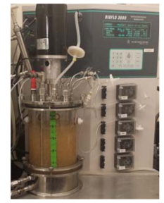
Figure 4 (above): Schematic of the semi-continuous culture operation method. Figure 5 (right): Transgenic rice cell culture grown in a 5 L bioreactor.
