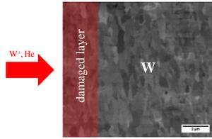
Ion-irradiation at the University of Surrey. The damaged layer is often in the micro-metre regime, depending on the type of ions and energy used
