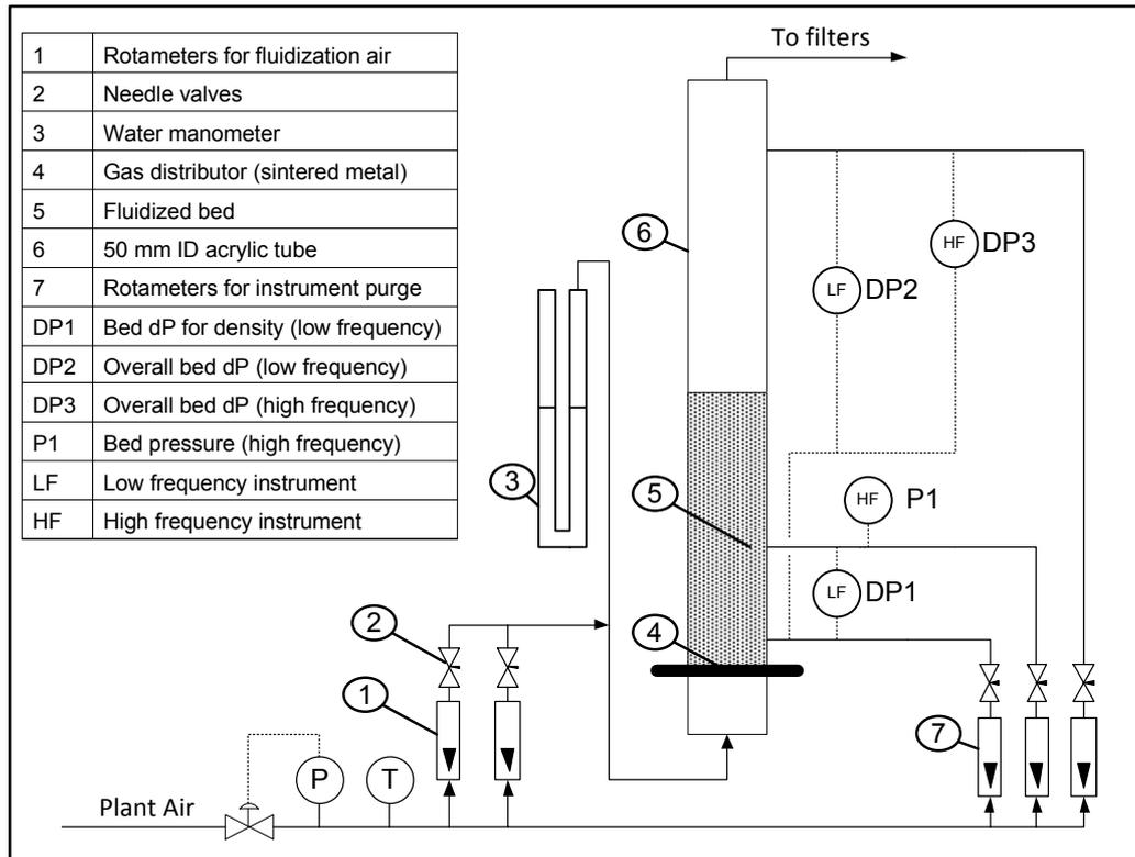
Figure 2: Experimental setup for cold model fluidization tests
