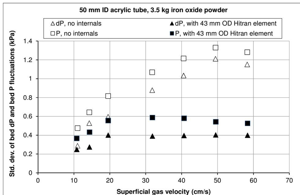
Figure 3: The effect of the Hitran element on the standard deviation of bed pressure drop and bed pressure fluctuations
