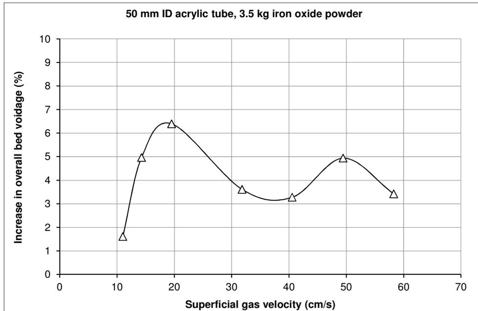
Figure 4: Percentage increase in the overall bed voidage with the Hitran element
