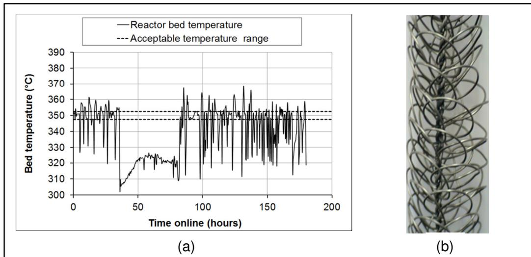
Figure 1: (a) Reactor bed temperature. (b) Hitran matrix element
