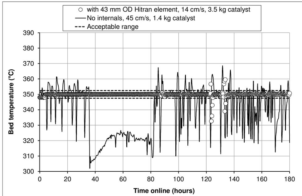
Figure 5: Reactor bed temperature with and without the Hitran element
