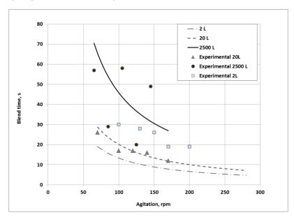
Figure 1 – Blend time design chart and experimental data for different bioreactor scales
