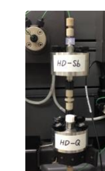
Tandem columns: Two devices stacked in series Top (HD-Sb); Bottom (HD-Q)
