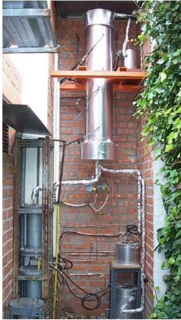
*Fig 2. Pilot Plant Reactor (SCWO) at the University of Valladolid*
