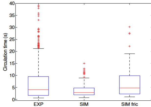
Figure-2. Box plot of the circulation time of fuel particles for the experimental data (EXP) and the simulation results neglecting (SIM) and considering the friction model (SIM fric). As can be seen, the friction model improves considerably the simulation results.
