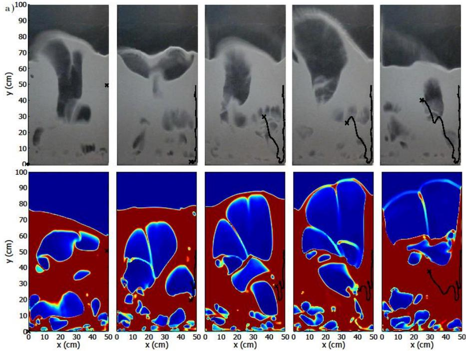
Figure-1. Path followed by a fuel particle in a 2-D fluidized bed obtained experimentally (upper row) and simulated with the hybrid-model (lower row). The path followed by the fuel particle in its sinking and rising process in a 2D fluidized bed showed qualitative good agreement between the experimental data and the simulation results.
