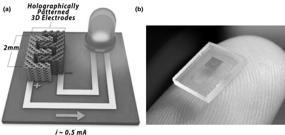
Figure 1 – (a) Schematic of a holographically defined lithium-ion microbattery, illustrating it lighting an LED with a 0.5 mA current which corresponds to a 600 C (~10 second) discharge. (b) Optical image of the holographically patterned microbattery on a glass substrate.
