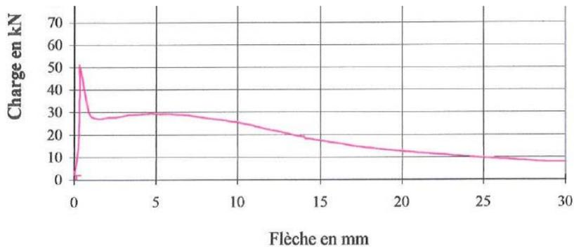
Figure 4: Unsatisfactory load-deflection curve in spite of 500J energy
