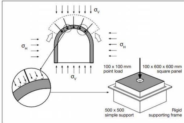
Figure 1: Sprayed concrete under flexural and shear load
