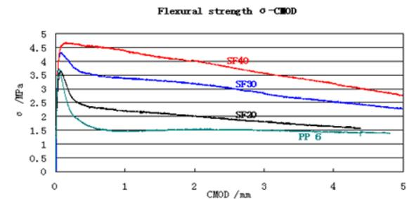
Figure 9: Comparison of flexural strength in the FRC compared to CMOD
