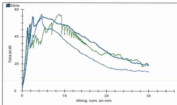
Figure 10: Dramix RC65/35BN 25kg/m<sup>3</sup> Curve load –deflection –Sigma report
