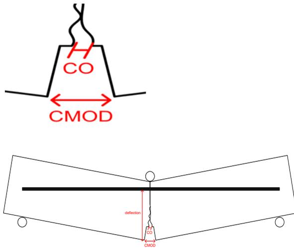
Figure 8: Definition of crack opening, CMOD and deflection
