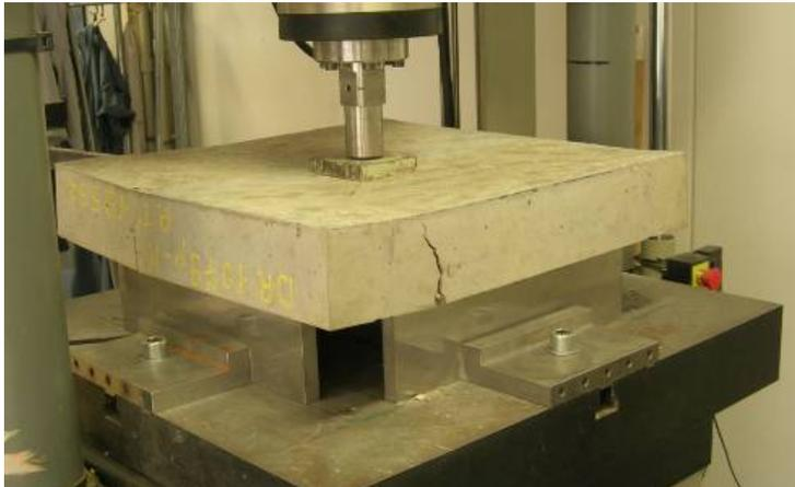
Figure 2: EN14488-5 Testing on steel support
