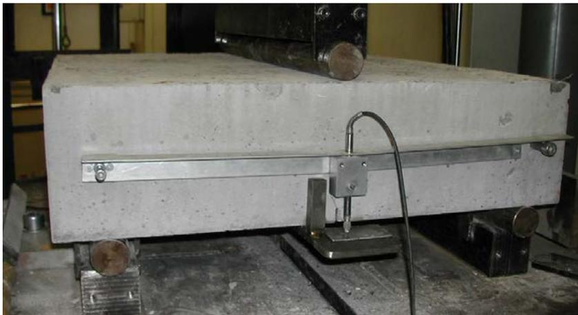
*Figure 6: Three point bending test on square panel with notch*
