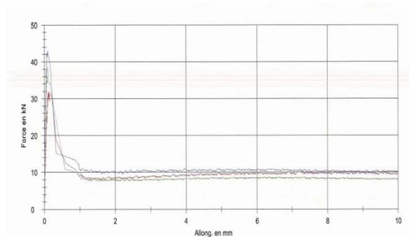
Figure 11: Curve Load –deflection with 6kg/m<sup>3</sup> macro-polymer fibre
