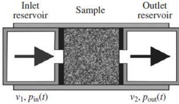
Figure 4: Transient pressure pulse test, Malkovsky [16].
