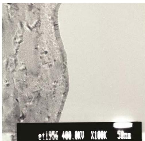
Figure 3: TEM micrograph of CTMSS membrane cross section
