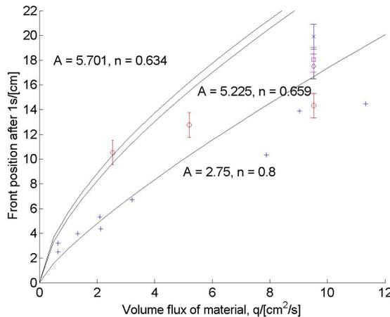
Figure 4. Front position after 1s as a function of the volume flux of material. Data from Eames & Gilbertson (6) (+) where  $u_{gi}/u_{mf} = 1.26$  is plotted along with our own data for ratios of 1.3 (O), 1.48 ( $\diamond$ ), 1.67 ([]), & 1.86 (x) respectively and lines corresponding to (11) for various values of  $A$  and  $n$ .
