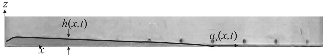
**Figure 1. Orientation of axes, and notation associated with modelling the currents. The image shows a fluidised current approximately 65cm long and 2cm thick. An outline has been drawn on the surface of the flow for clarity**
