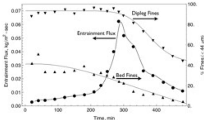
$\rho_p=2300 \text{ kg/m}^3$ ,  $d_{p50}(\text{initial})=57 \mu\text{m}$ , Bed Height=1.3 m
