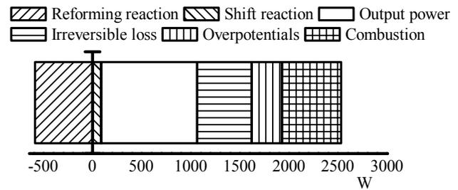
Figure 4 Energy generation in a system.
