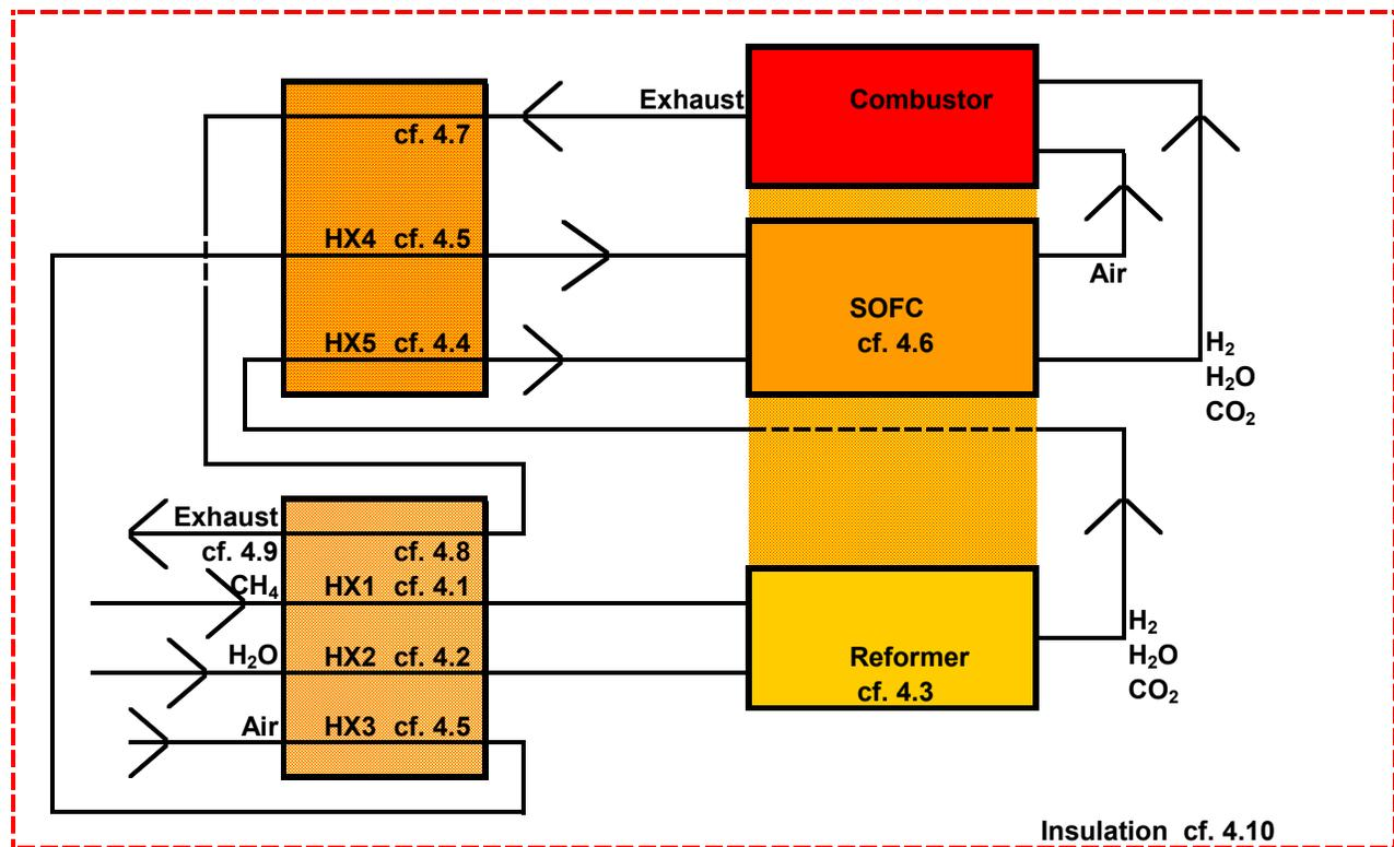
Figure 1 Simplified model of SOFC system.
