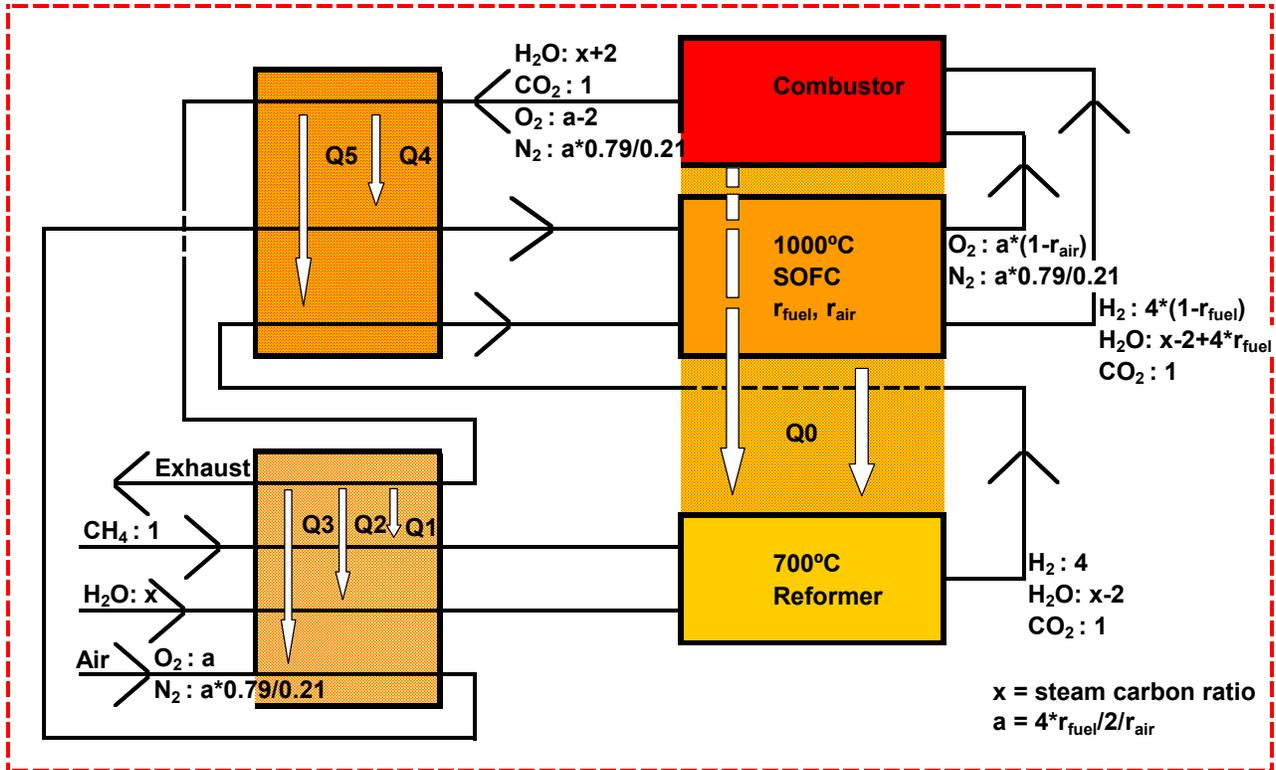
Figure 2 Mass (mol) balance of SOFC system.
