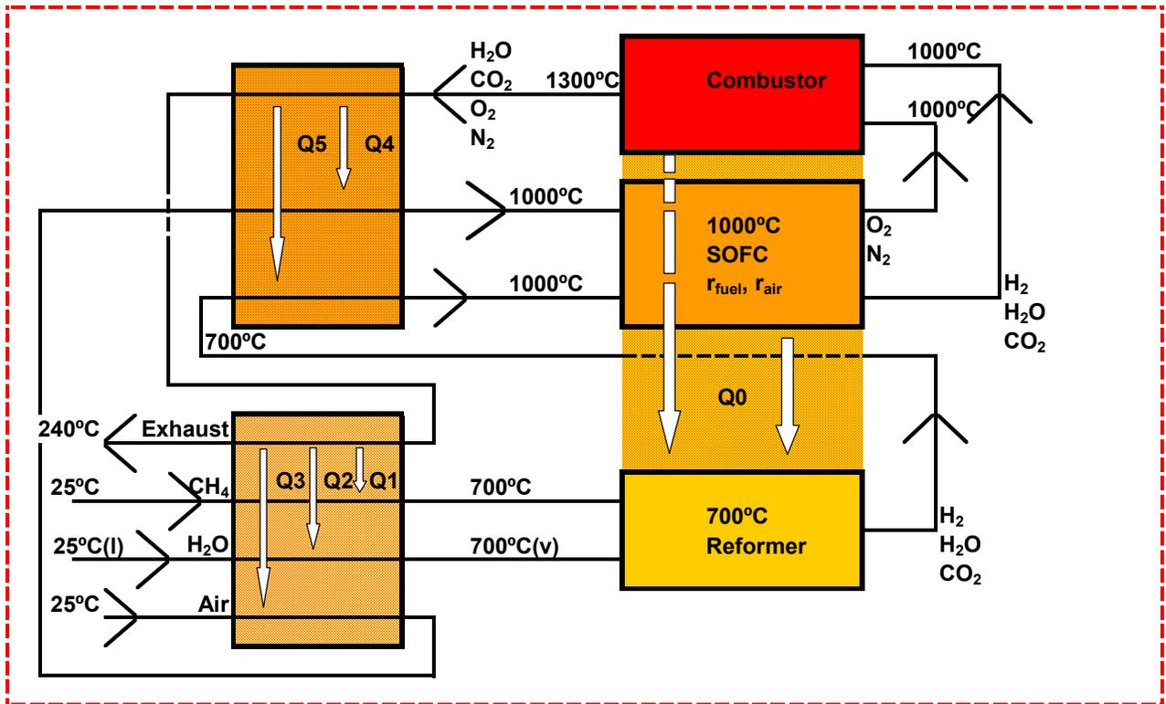
Figure 3 Energy balance of SOFC system.
