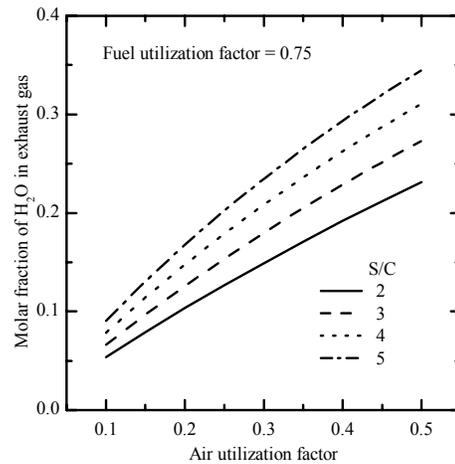
Figure 6 Molar fraction of  $\text{H}_2\text{O}$  in exhaust gas.
