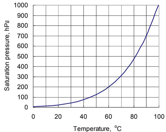
Figure 8 Temperature vs saturation pressure of water (Dew point vs partial pressure of steam vapor).
