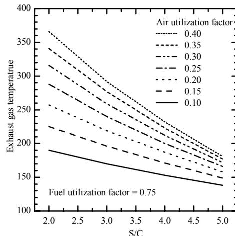
Figure 7 Exhaust gas temperature estimated for fuel utilization factor 0.75.
