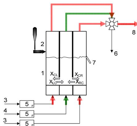
Figure 1. Schematic diagram of three partitioned fluidized bed apparatus
