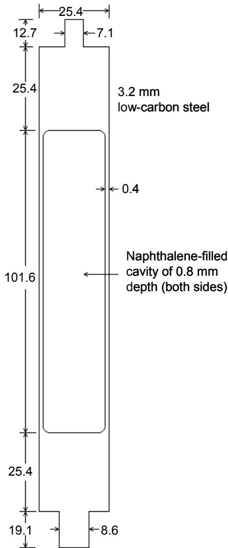
**Figure 2. Fins used in naphthalene sublimation experiments. All dimensions in mm.**
