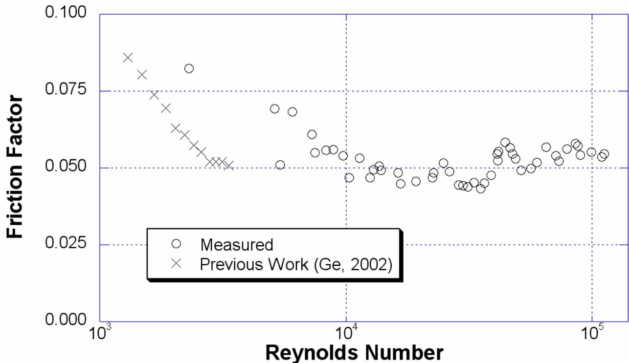
Figure 3. Friction factor,  $f$ , of the offset-strip fin array as a function of Reynolds number. Low Reynolds number data from previous work is included for comparison.
