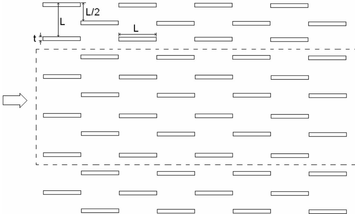
**Figure 1.** The scaled-up offset strip fin array under investigation. The array height (into the page) was 152 mm,  $L=25.4$  mm, and  $t = 3.18$  mm. The fins within the dotted box were used for measurements in the naphthalene sublimation experiments.
