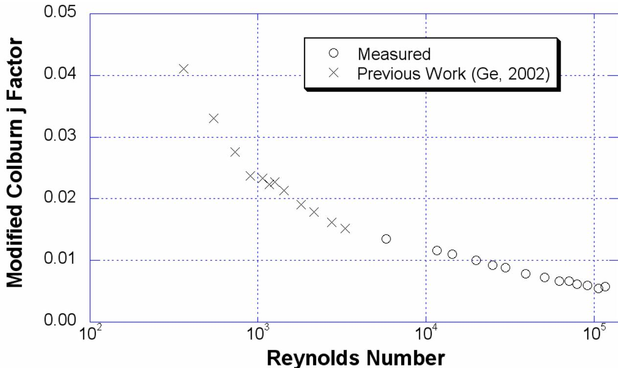
Figure 4. Modified Colburn  $j$  factor of the offset-strip fin array as a function of Reynolds number. Low Reynolds number data from previous work is included for comparison.
