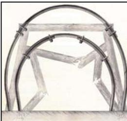
Picture 3: timber cribs and yieldable steel support
