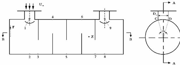
Fig. 2 Shell-and-tube HEx with normal baffles
