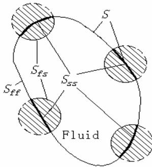
Fig. 1 Sample control volume with tubes
