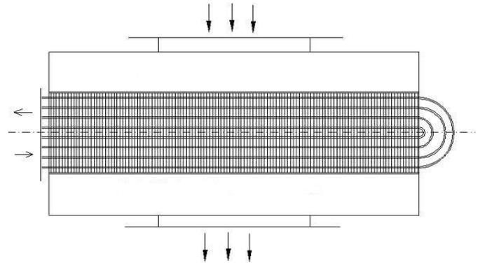
Fig. 19 Two-pass arrangement of water side
