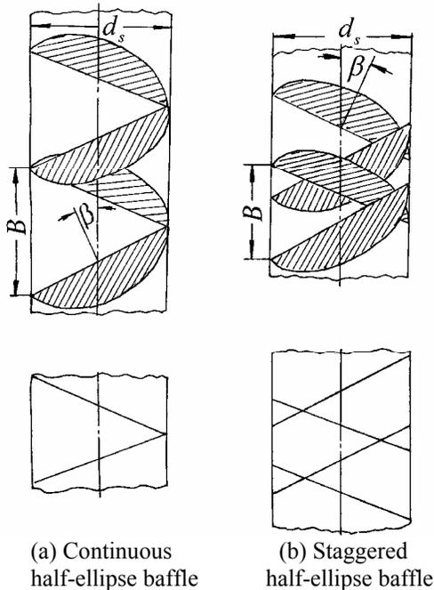
Fig.12 Half-ellipse helical baffles
