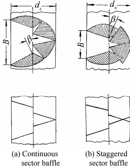
Fig.13 Sector helical baffles
