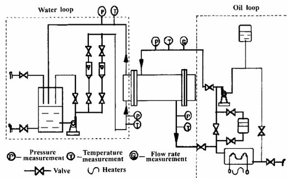
Fig. 16 Test system for heat transfer measurement
