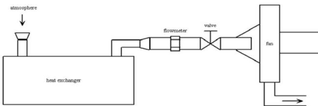
Fig. 10 Test apparatus for S-T HEx with vertical baffles
