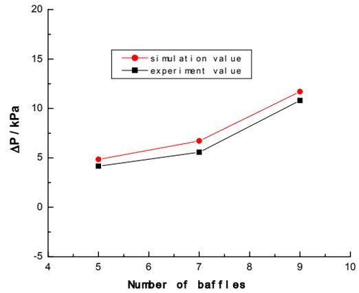
Fig.11 Effect of baffle number on the total pressured drop
