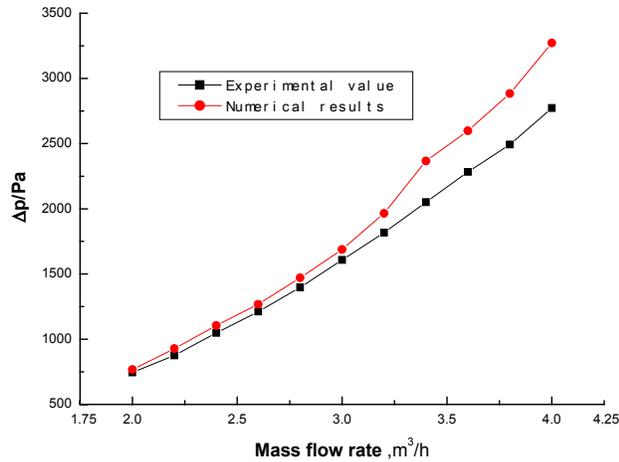
Fig. 17 Variation of pressure drop with mass flow rate
