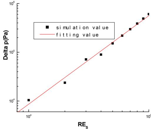
Fig. 6 Shell side pressure drop vs.  $Re_s$
