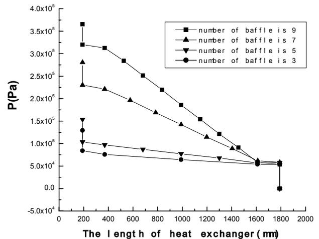
Fig. 8 Effect of baffle number on fluid pressure drop
