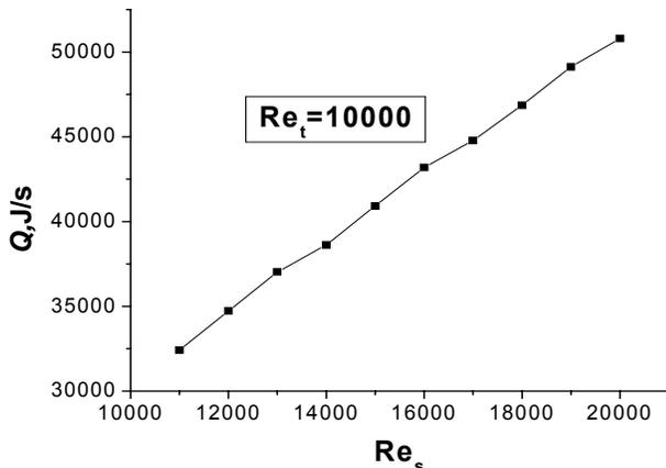
Fig. 23 Variation of heat transfer rate with shell side Re
