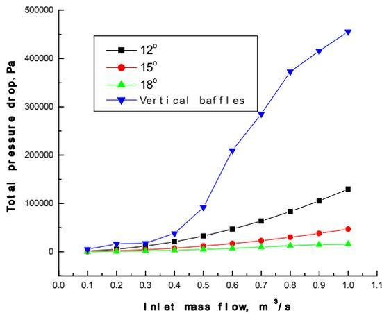
Fig. 15 Effect of helical angle on the pressure drop
