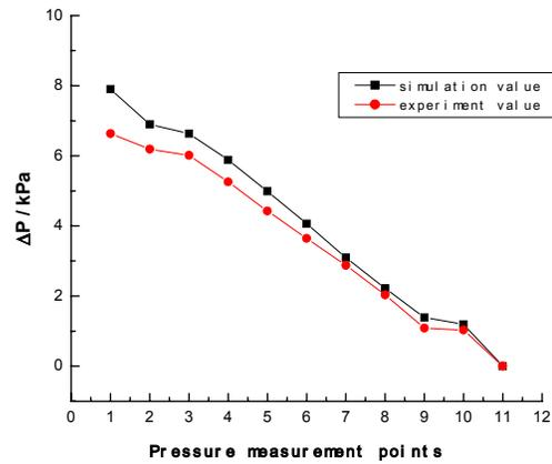
(b) Mass flow rate =  $0.26 \text{ m}^3 / \text{s}$
