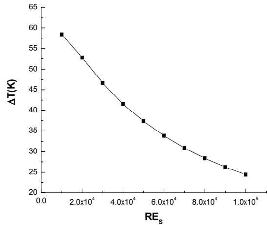
Fig. 7 Effect of  $Re_s$  on shell side temperature difference
