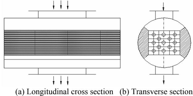
Fig. 18 Shell-and-tube heat exchanger with finned tube bank
