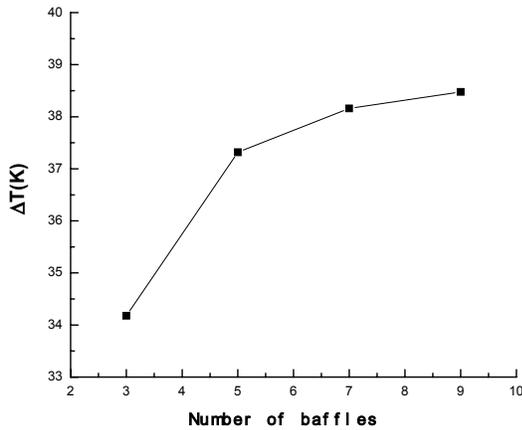
Fig. 9 Variation of shell side  $\Delta T$  with baffle number
