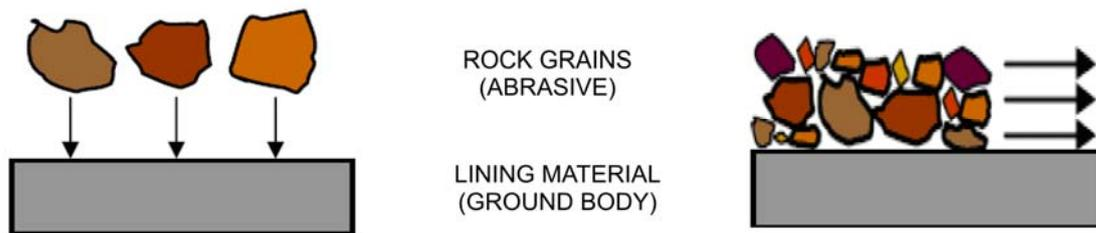
Fig. 14: Types of wear on the lining material
