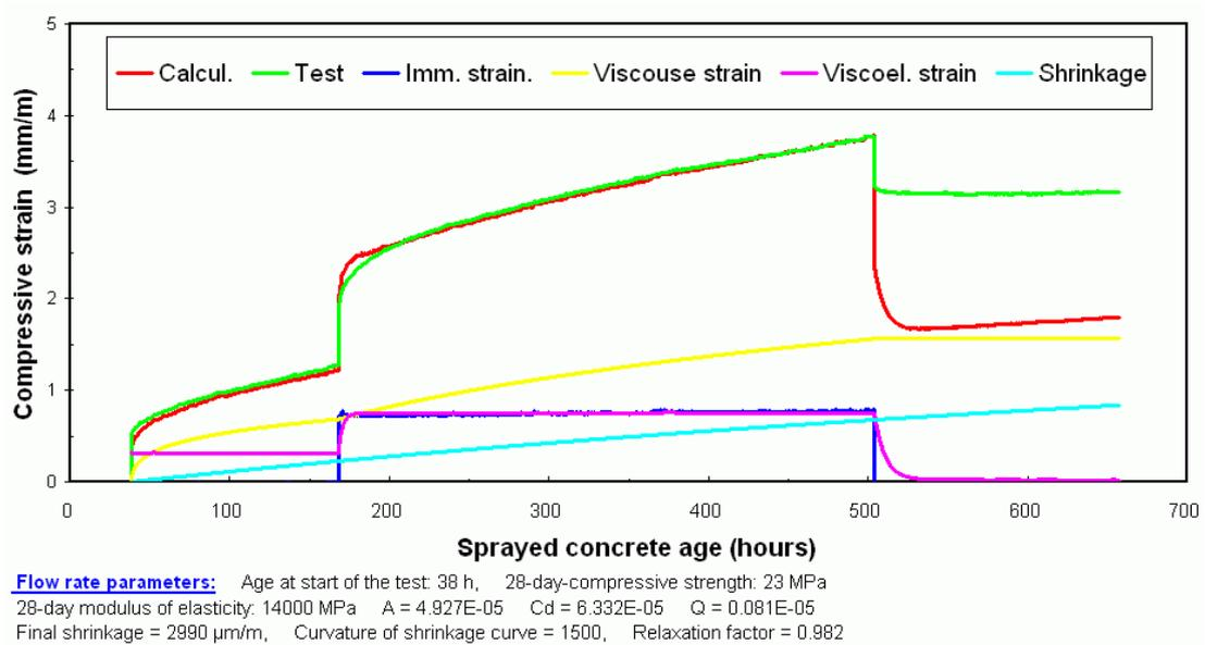
Fig. 8: Flow rate parameter identification for the average value curve for longitudinal compressive strain
