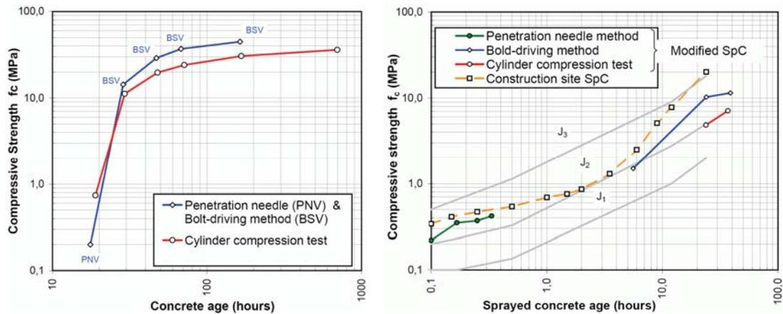
Fig. 3: Early strength development evaluated by means of penetration needle and bold-driving methods and cylinder compression tests.
