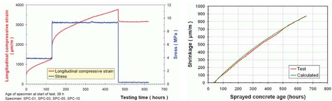
Fig. 7: Average value curves of the a) longitudinal compressive strain and stress and b) shrinkage strain
