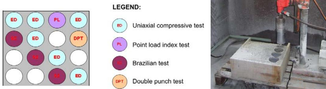
Fig. 16: Sampling in the laboratory.
