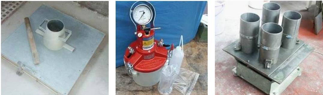
Fig. 1: a) Flow table, b) Air meter c) Cylindrical steel forms
