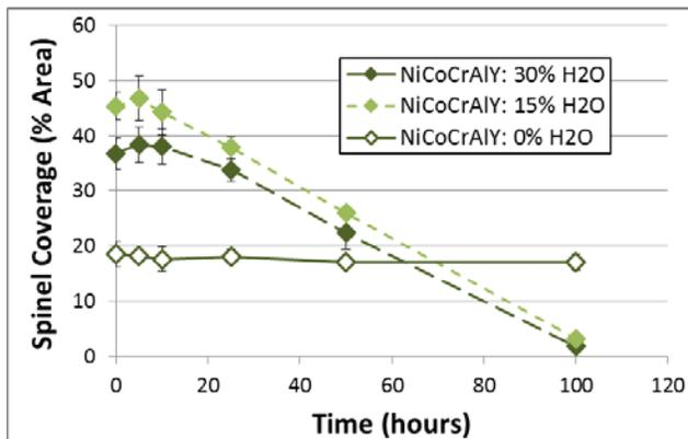
Figure 1 – Spinel surface area coverage versus time for NiCoCrAlY specimens oxidized in 30, 15 and 0%  $H_2O$ .
