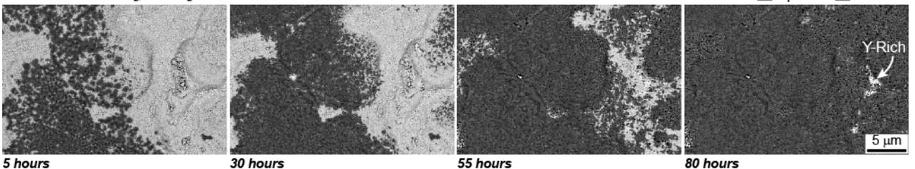
Figure 2 – A “timelapse” of NiCoCrAlY TGO (20%  $O_2$ , 15%  $H_2O$ ) from 5 to 80 hours. All backscatter images (5kV) were taken at the same site with 25 hours of oxidation (plus ramping times) separating them.
