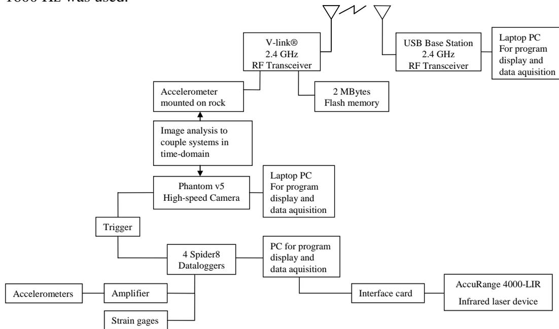
Figure 4: Schematic layout of data acquisition system.
