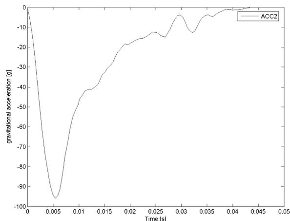
Figure 6: Typical deceleration history of low-energy rockfall impact.
