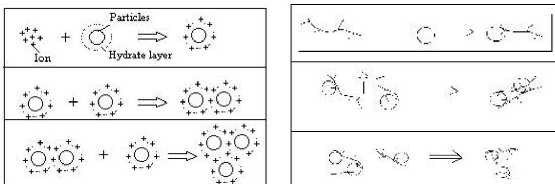
Figure 3: Physical models of Coagu-flocculation process
