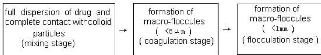
Figure 2: Coagu-flocculation process
