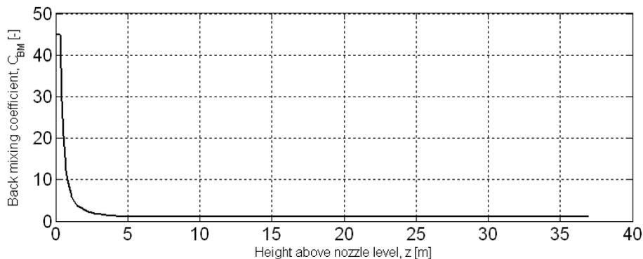
Figure 5. The back mixing coefficient along the centerline of the furnace for the 330 MW<sub>th</sub> CFB investigated in this work.
