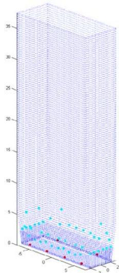
Figure 3. The 330 MW<sub>th</sub> CFB furnace geometry as implemented in the modeling.
