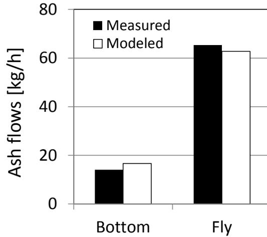
Figure 4. Bottom and fly ash flows in the Chalmers 12 MW<sub>th</sub> CFB boiler – measured and modeled.
