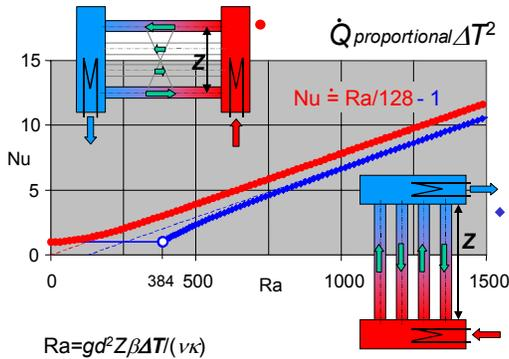
**Fig. 6.** Nusselt vs. Rayleigh numbers for natural convection in horizontal (upper curve) and vertical (lower curve) tube bundles with adiabatic walls.
