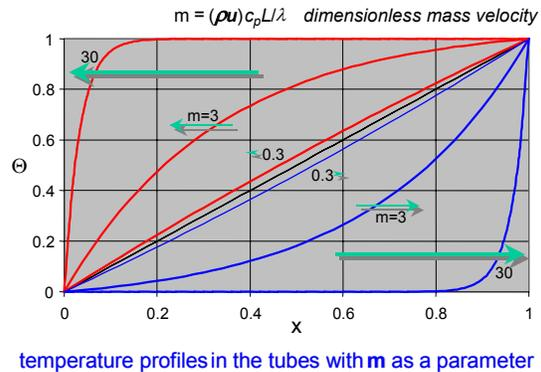
**Fig. 5** Temperature profiles in the channels of tube bundles (see Fig. 4) in natural convection as a function of flow rate  $m$
