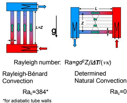
**Fig. 4** Natural convection in tube bundles.
