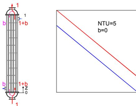
**Fig. 8.** Temperature distribution without backflow in a vertical shell-and-tube heat exchanger – ideal counter flow.
