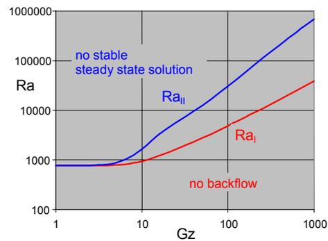
**Fig. 10** Nickolay's stability chart for laminar mixed convection in vertical tube bundles.
