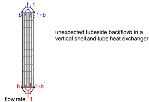
**Fig. 7.** Unexpected tubeside backflow in a vertical shell-and-tube heat exchanger
