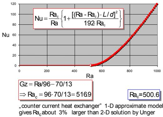
**Fig. 3** Approximate solution to the natural convection problem in a single vertical parallel plates channel.
