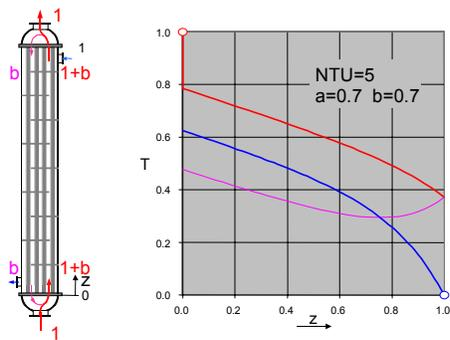
**Fig. 9.** Temperature distribution with backflow in a vertical shell-and-tube heat exchanger
