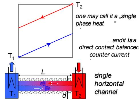
**Fig. 1** Natural Convection in a Single Horizontal Channel.
