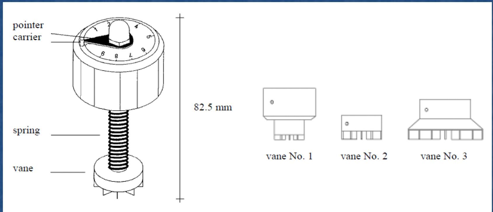
Pocket vane shear apparatus
