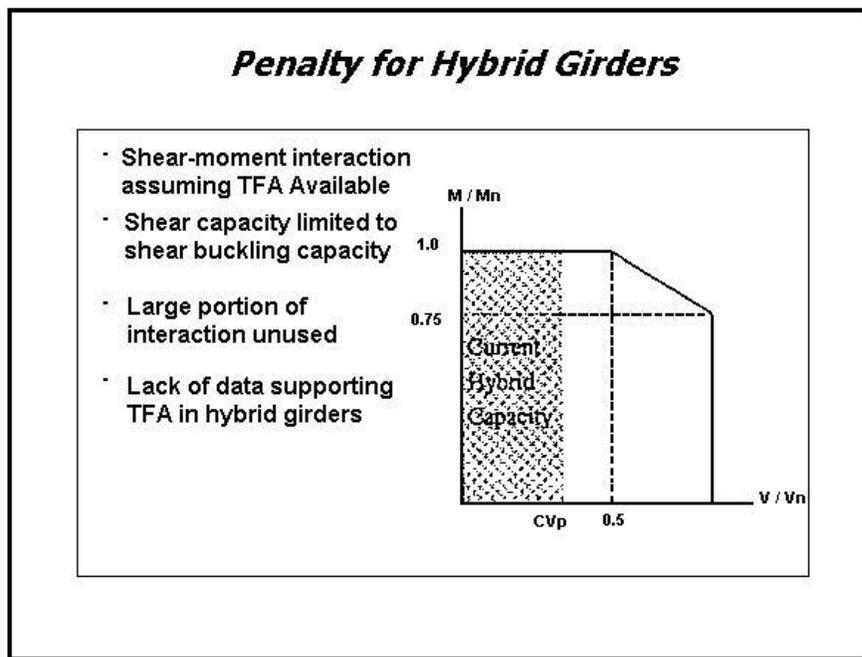
Figure 4. Hybrid Girders and Tension-Field Action
