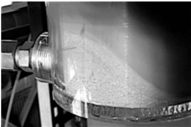
Figure 3: Still shots from a video of the 7.6-cm (3-inch) ID cylindrical jet cup with a 0.48-cm (0.1875-inch) diameter nozzle at a gas velocity of 137 m/sec (450 ft/sec).
