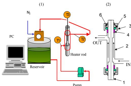
**Figure 3. Alcor HLPS system(1) and heater section(2).**
