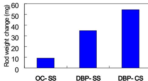
**Figure 10. HLPS test of DBP.** Experimental conditions: same as Figure 5. OC-SS: additive -OC, rod material-stainless steel 304, DBP-SS: additive-GBL, rod material-stainless steel 304, DBP-CS: additive-GBL, rod material-carbon steel.
