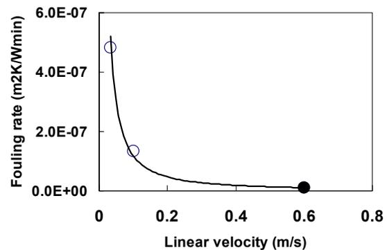
**Figure 12. Liner velocity effect.** Experimental conditions are described in the caption of figure 11. Open circle:  $Q=13,000\text{-}19,000 \text{ w/m}^2$ , Fouling rate of linear velocity 0.6m/s at the low heat flux ( $Q=13,000 \text{ w/m}^2$ ) is zero for 5 hours. Solid circle:  $Q=180,000 \text{ w/m}^2$ .
