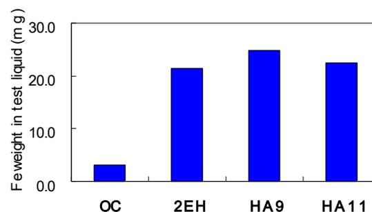
**Figure 6. Fe weight in the test liquid after experiment.** Experimental conditions: same as figure 5. Liquid volume of each experiment is about 300 ml. Before experiment, the Fe weight was about 3 mg in the test liquid.
