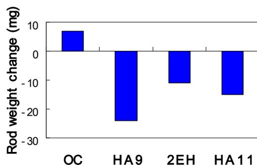
**Figure 5. Fouling rate test for higher alcohols.** Experimental conditions; Outlet bulk liquid temperature 140°C, pressure 0 MPaG (vapor ratio=0), run time 15 hours, heater rod material: carbon steel.
