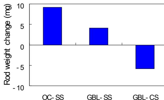
**Figure 9. HLPS test of GBL.** Experimental conditions: same as Figure 5. OC-SS: additive=OC, rod material=stainless steel 304, GBL-SS: additive=GBL, rod material=stainless steel 304, GBL-CS: additive=GBL, rod material =carbon steel.
