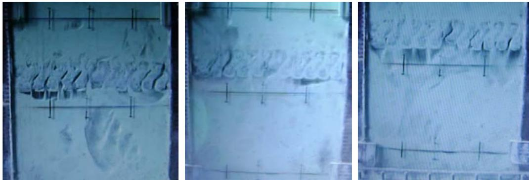
Figure 2. Role of additional distributor in bubble braking
