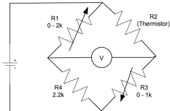
**Figure 1 Thermistor bridge**
