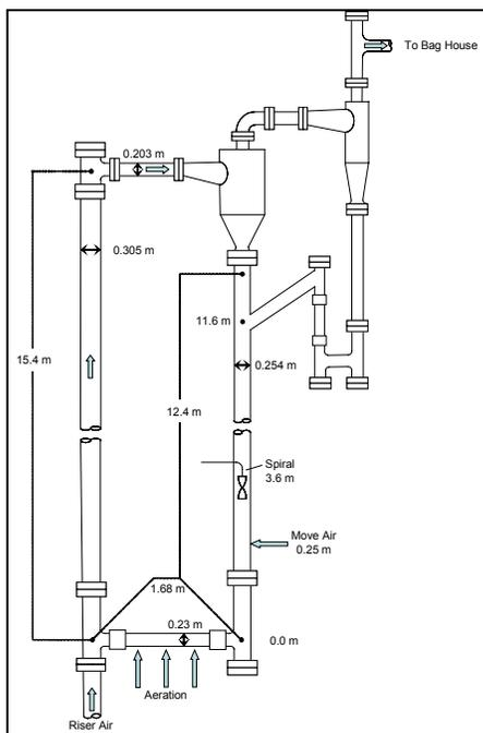
**Figure 4 Schematic Diagram of CFB Test Unit**
