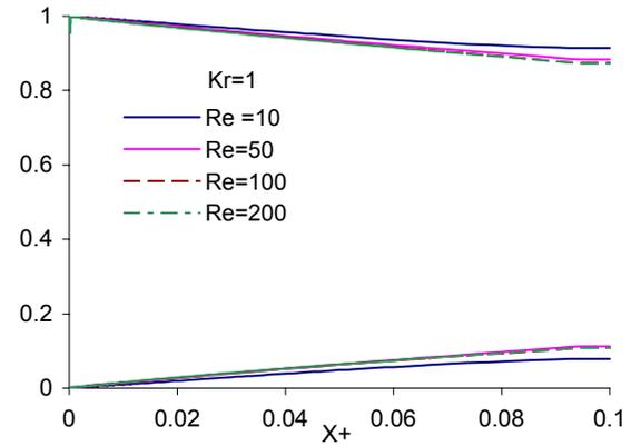
Figure 2 Longitudinal variation of the hot and cold fluid mean temperature
