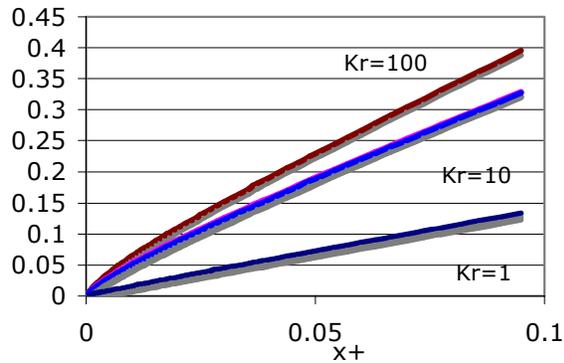
Figure 5 Variation of the Average NTU along balanced parallel flow heat exchanger ( $\alpha=1$ )
