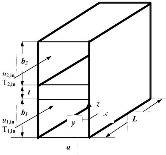
Figure 1 Three-dimensional sketch of the rectangular duct parallel flow heat exchanger
