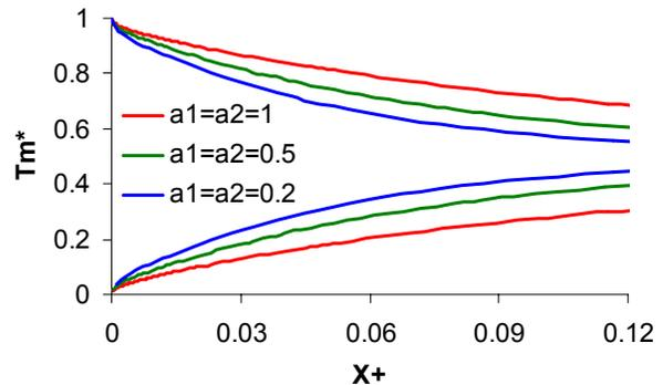
Figure 3 Longitudinal variations of the mean temperatures of hot and cold fluids for  $K_r=100$
