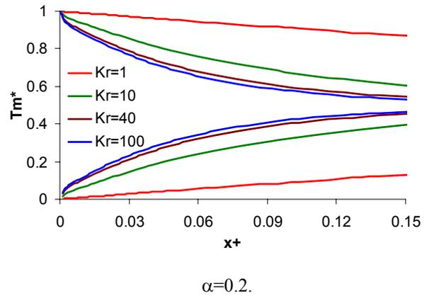
Figure 4 Longitudinal variations of the mean temperatures for rectangular ducts
