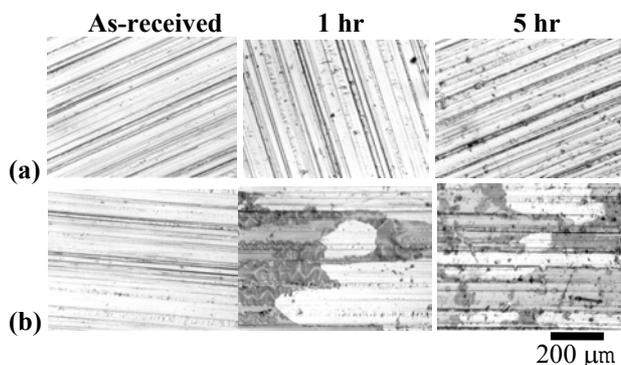
Fig. 6 Optical microscope photographs of plasma polymers at (a) anode and (b) cathode electrode with boiling time.
