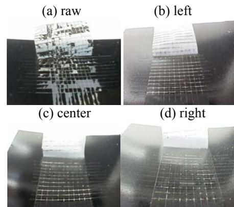
Fig. 11 Results of tape peel test for paints on OPZ treated Al at different places.
