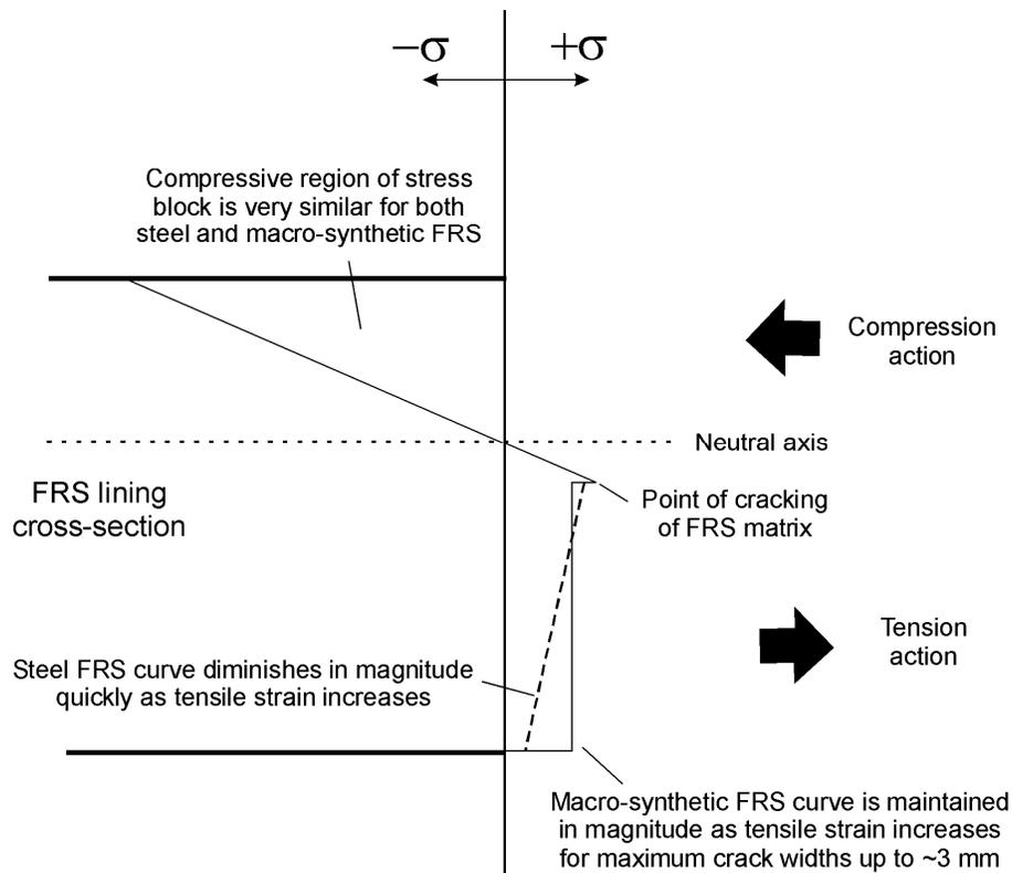
Figure 3. Stress distribution through a FRS lining subject to flexure and reinforced with steel or synthetic fibres.
