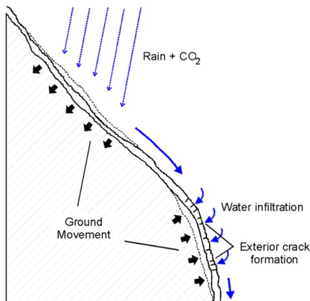
Figure 1. Crevice corrosion of steel fibres and bars on a slumping slope.
