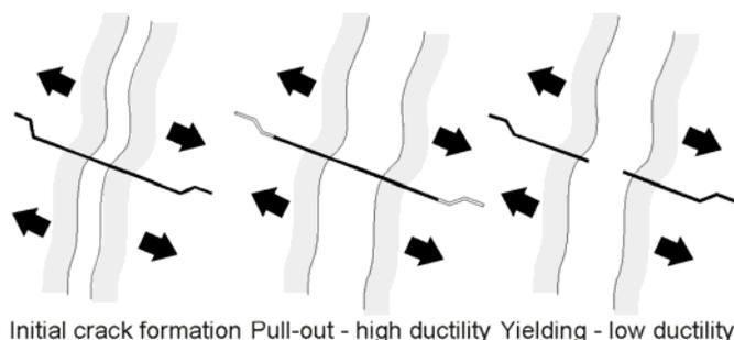
Figure 2. Post-crack failure mechanisms for FRS reinforced with steel fibres.
