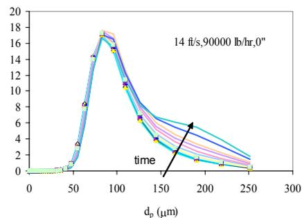
Figure 6. Particle size distribution in the riser as a function of time after the solids cutoff transient.
