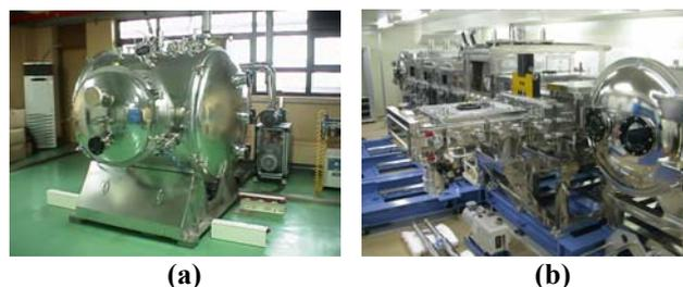
Fig. 14 Photographs of IAR mass production systems: (a) batch type and (b) roll to roll type.
