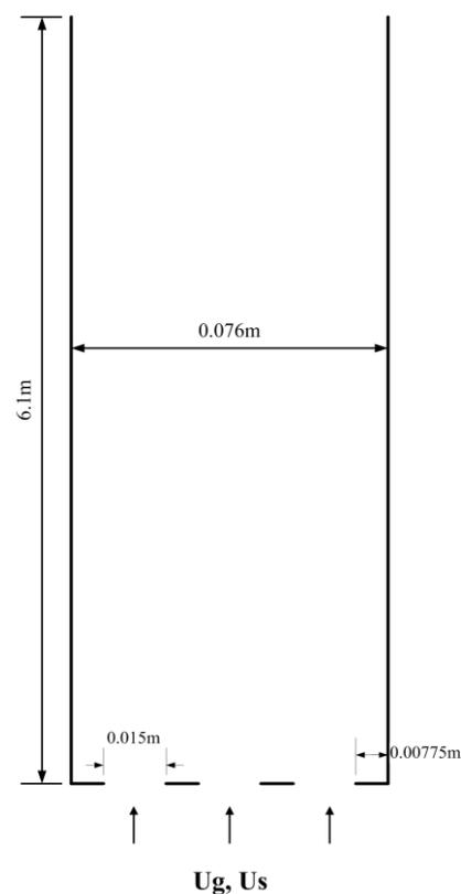
Figure 1. Schematic diagram of the 2-D riser
