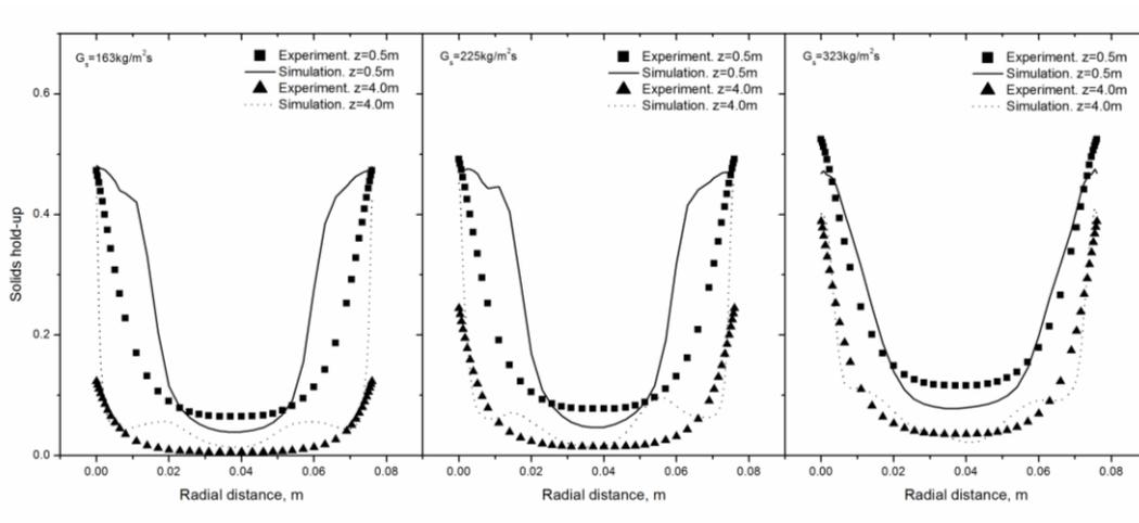
Figure 3 Comparison of time-averaged radial solid concentration profiles at two heights predicted by EMMS-based two-fluid model with experimental data under different solid fluxes
