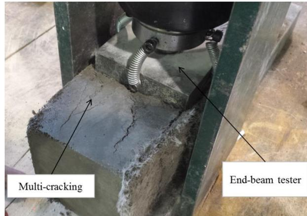
**Figure 4: Hardened specimen tested in compression at 1 hour using end-beam tester**
