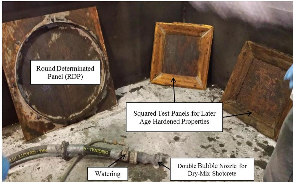
**Figure 1: Shotcrete nozzle and test panels used to produce shotcrete specimens**
