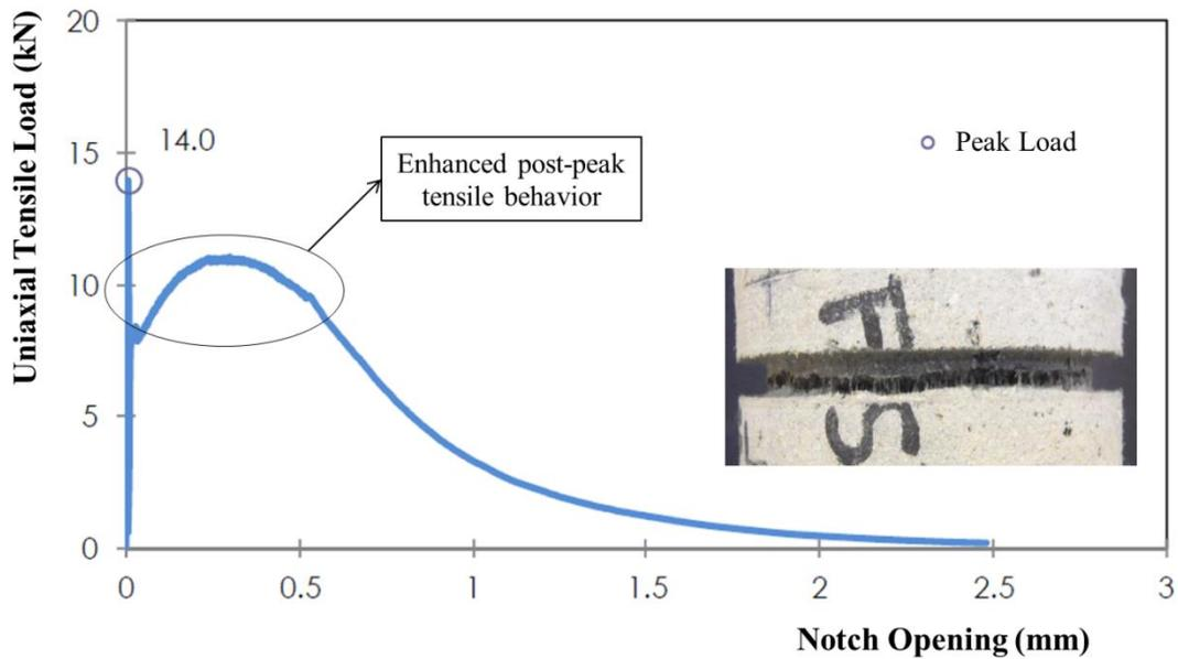
**Figure 5: Uniaxial tensile load curve versus notch opening obtained at 28 days shotcrete cores**
