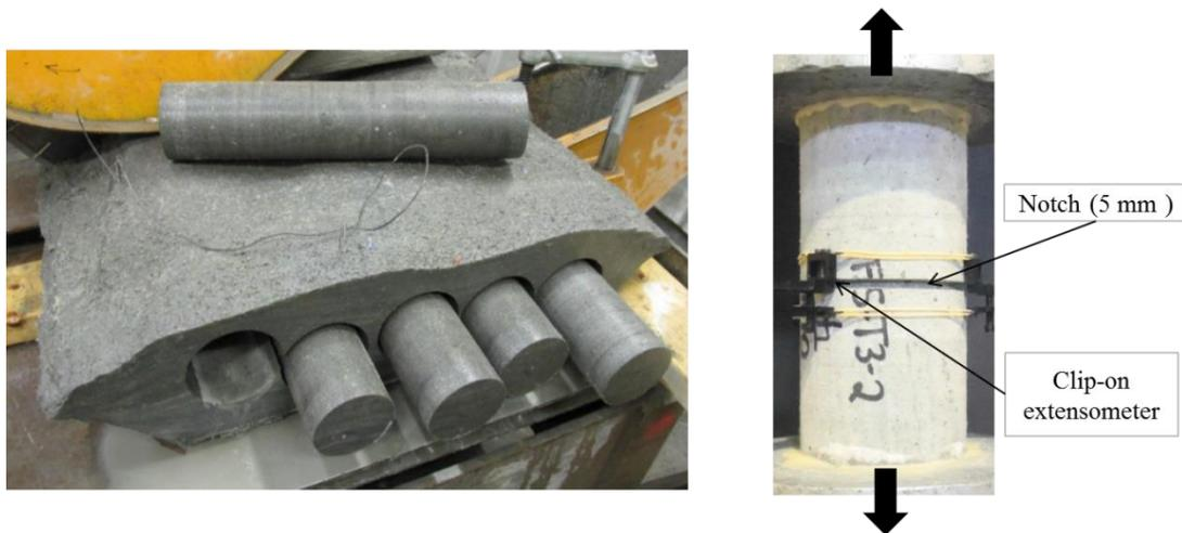
**Figure 3: Shocrete cores extracted from test panel (left) and tested for direct tensile strength evaluation (right)**
