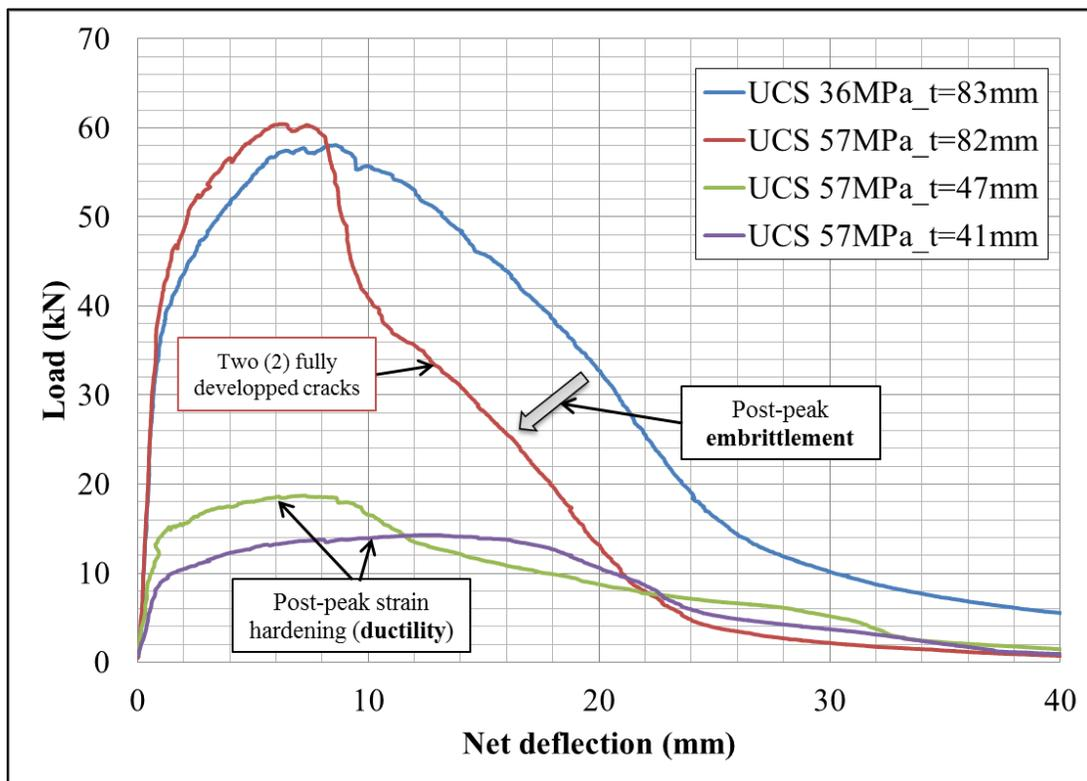
**Figure 6: Post-peak embrittlement observed on 80 mm thick RDP panels and Post-peak strain hardening ductility observed on 40 mm thick RDP panels tested according to the ASTM C1550**
