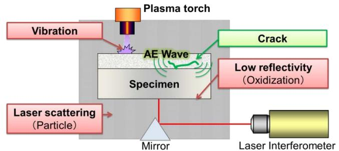
Fig.2 Schematic of laser AE measurement during plasma spraying<sup>(3)</sup>.
