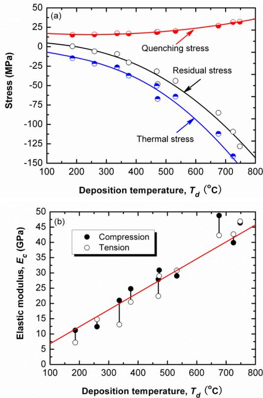
Fig.1 (a) Residual stresses in and (b) elastic modulus of plasma sprayed TBC formed at different deposition temperatures<sup>(1,2)</sup>.
