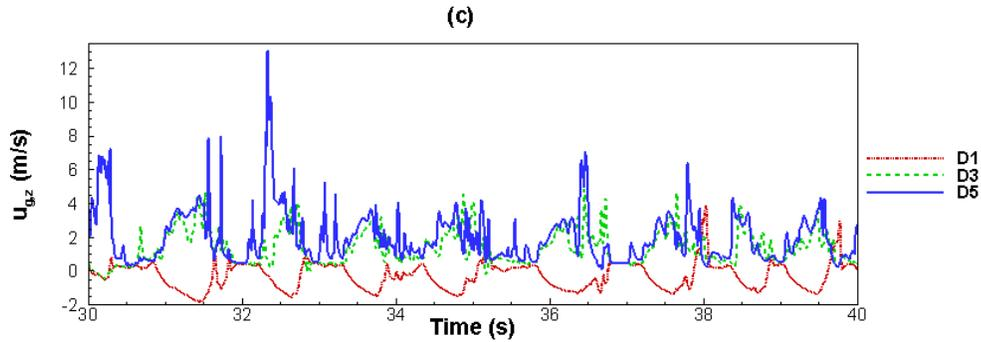
Figure 3. (a) tracer concentration, (b) voidage, and (c) gas velocity versus time at different downstream sampling points.
