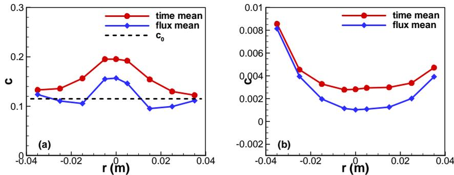
Figure 6. Flux-based mean concentration and time-average concentration (a) downstream ( $z = 1.3$  m) and (b) upstream ( $z = 0.8$  m).
