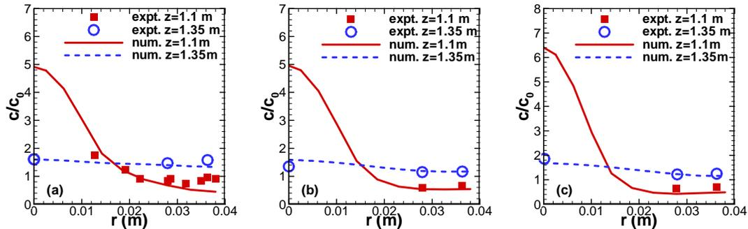
Figure 1. Radial profiles of mean tracer concentration above the injection level for  $U_g =$  (a) 0.183 m/s; (b) 0.274 m/s; (c) 0.354 m/s and experimental data from (9).
