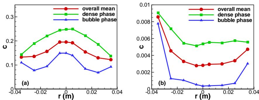
Figure 5. Profiles of mean tracer concentration and concentrations in bubble and dense phases (a) downstream ( $z = 1.3$  m) and (b) upstream ( $z = 0.8$  m).
