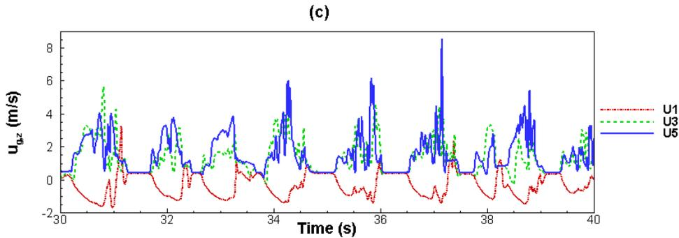
Figure 4. (a) tracer concentration, (b) voidage, and (c) gas velocity versus time at different upstream measuring points.
