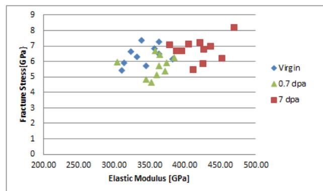
Figure 2 – Scatter plot showing increase in elastic modulus with implantation damage
