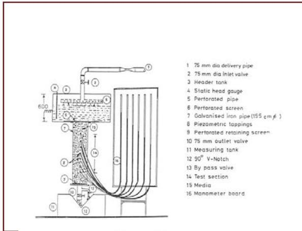
Fig : Parallel flow permeameter
